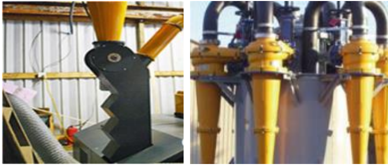
Fig. 29. Zig-Zag Separator (Dry-Gravity Process) (Left) Cyclone Separator (Wet-Gravity Process) (Right)
