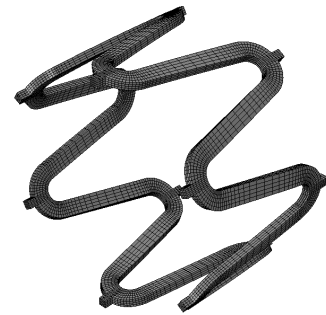
(b) Stent geometry with increased strut thickness.
